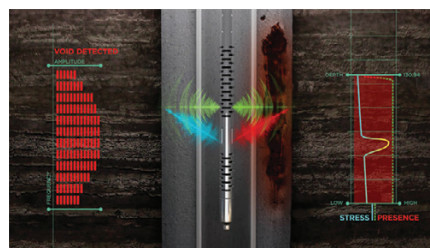
Enhanced discrimination of cement defects.
